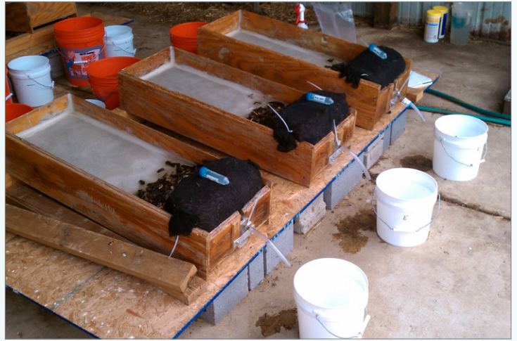
Filtrexx lab testing for EnviroSoxx performance.
