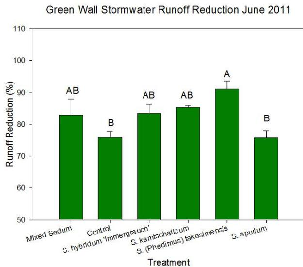
Figure 6c. Percent reduction in runoff for each treatment in June 2011. Bars with different letters are significantly different within figure ( $\alpha < 0.1$ ).
