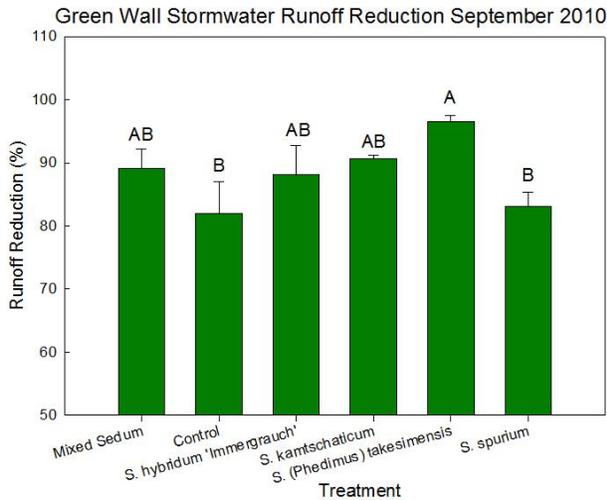
Figure 6a. Percent reduction in runoff for each treatment in September 2010. Bars with different letters are significantly different within figure ( $\alpha < 0.1$ ).
