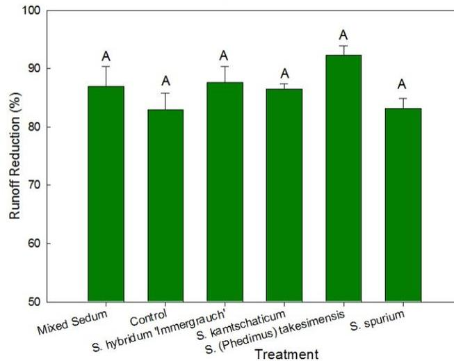
Figure 5a. Percent reduction in runoff for study period (8-10/10, 3-6/11). Bars with different letters are significantly different within figure ( $\alpha < 0.1$ ).
