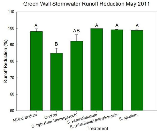
Figure 6b. Percent reduction in runoff for each treatment in May 2011. Bars with different letters are significantly different within figure ( $\alpha < 0.1$ ).
