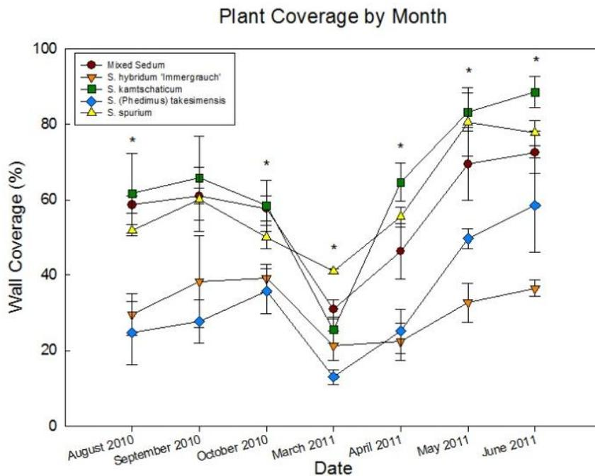
Figure 3b. The percent wall coverage for each treatment during the months for which both coverage and stormwater were measured. An asterisk indicates a difference between one or more means ( $\alpha < 0.05$ ; Error Bars represent  $\pm 1$  SE)
