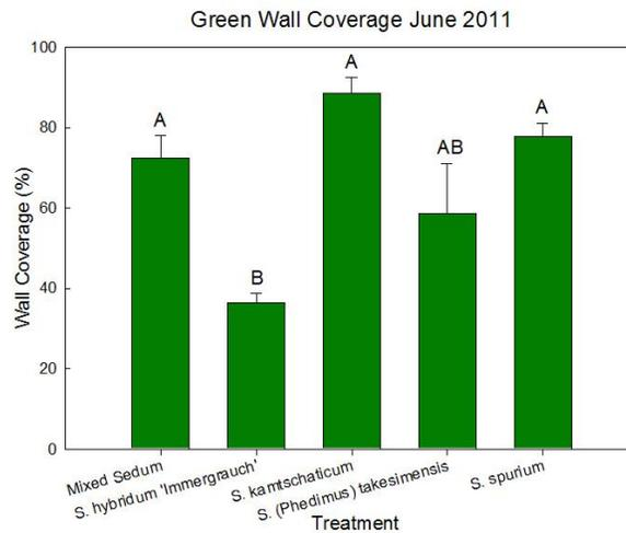
Figure 4c. Percent plant coverage on June 2011. Bars with different letters are significantly different within figure ( $\alpha < 0.05$ ).
