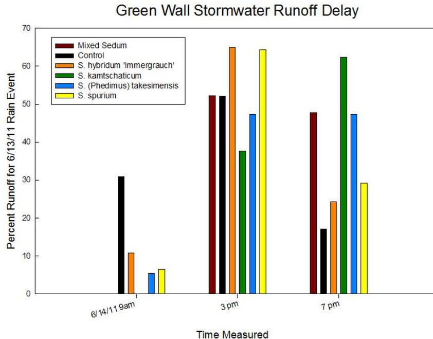
Figure 7b. Percent runoff volume discharged at 9 am, 3 pm, and 7 pm on 6/14/11.
