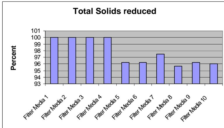
**Figure 2:** Percent of motor oil in runoff removed by compost filter media, n=7.
