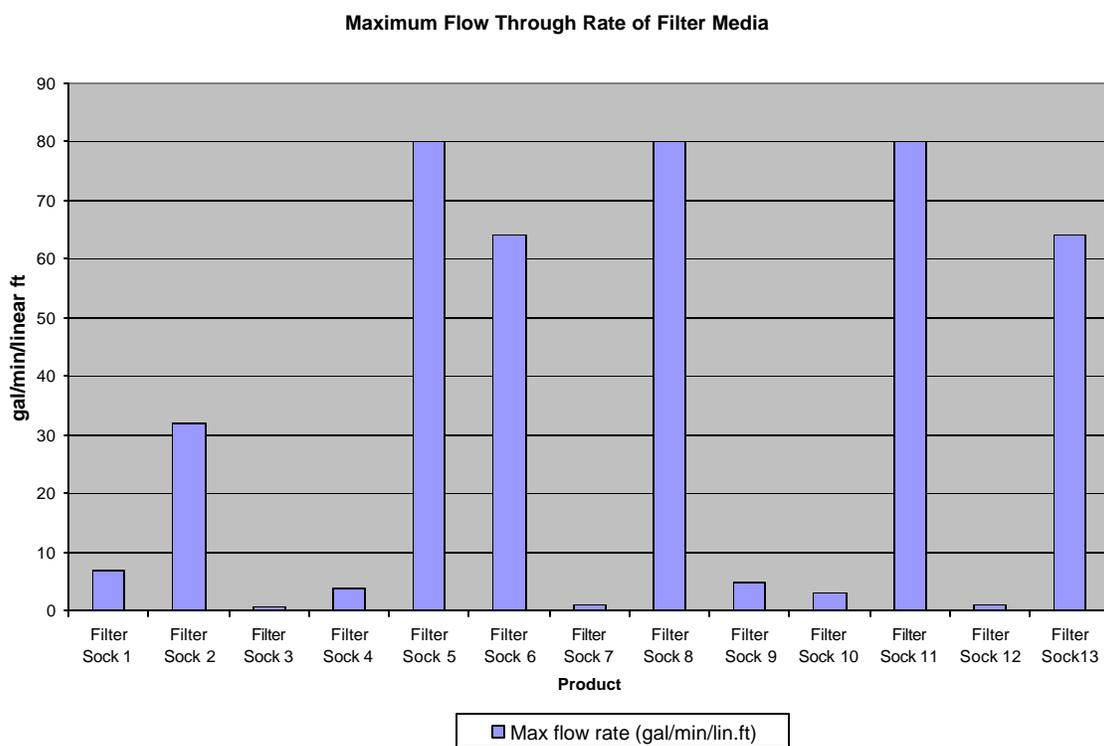
**Figure 3:** Maximum recorded flow through rate and moisture content of filter media.
