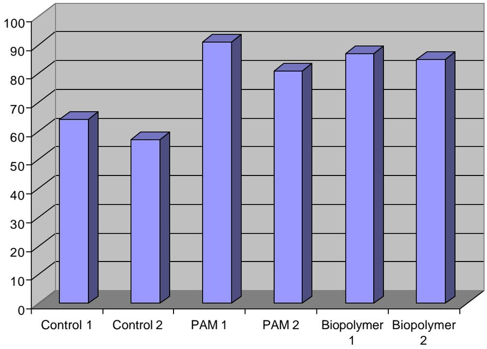
Figure 4--Soluble P removal efficiency from storm water runoff with polymer added to filter sock.
