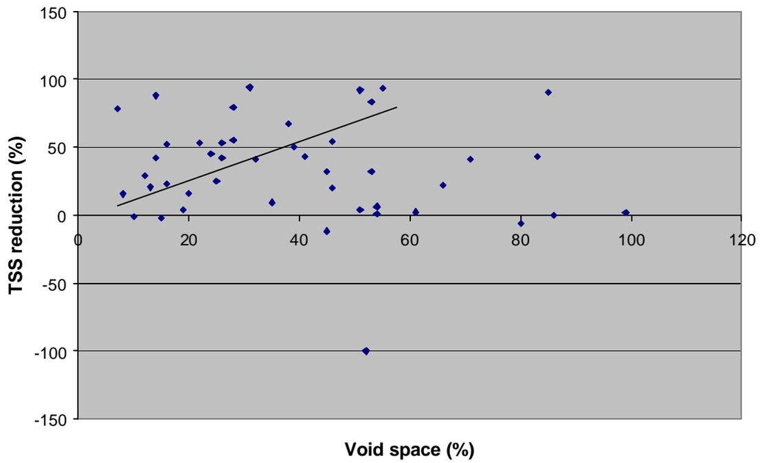
Figure 13--Void space of filter media relative to turbidity reduction in runoff.
