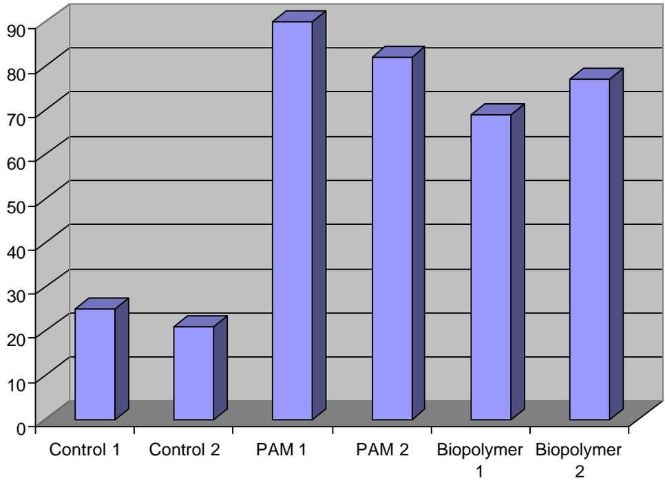
Figure 3--Percent TSS removal efficiency from two consecutive runoff events with polymer added to filter socks.
