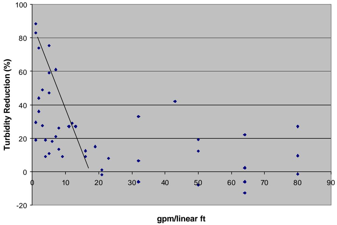
Figure 7--Hydraulic flow through rate of filter media relative to motor oil removal efficiency in runoff.
