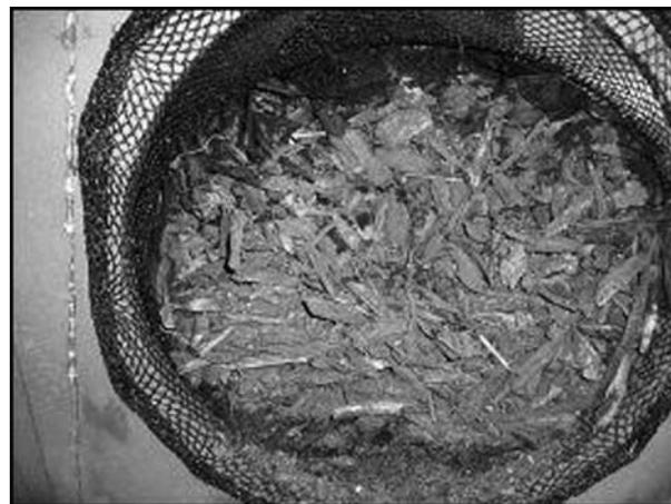
Fig. 3. Filling of 30.5-cm diam. (12 in) SiltSoxx with coarse material.
