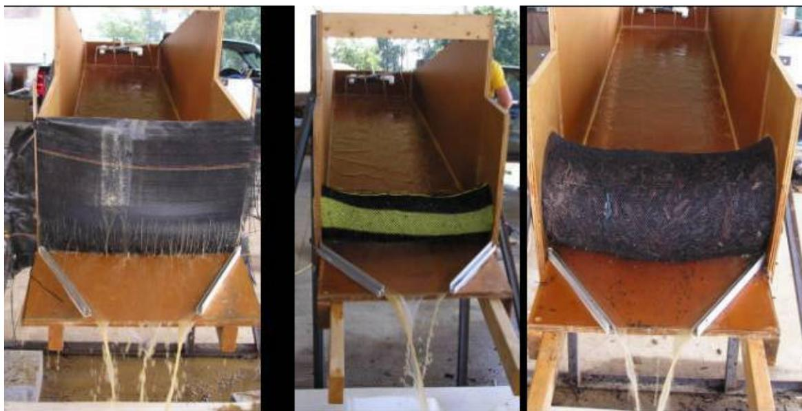
Figure 5. Flow of sediment-laden runoff through sediment control devices at 2 gpm at 10 minutes time. From left to right, 24 in. silt fence (mounted with 18 in. above flume bottom), 8 in. coarse SiltSoxx™, and 12 in. coarse SiltSoxx™.
