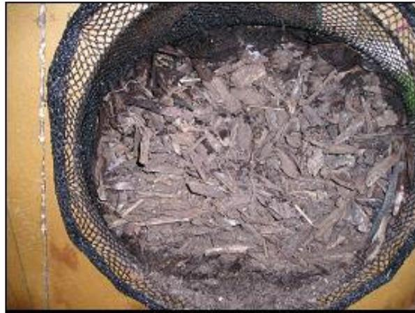
Figure 3. Filling of 12 in. SiltSoxx™ with coarse material.
