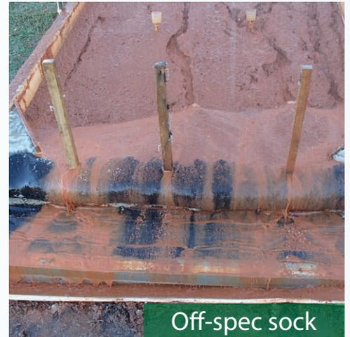
Devices with low flow-through rate, such as off-spec filter sock, overtop faster due to increased ponding & hydraulic pressure behind the device.
