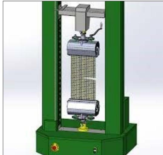
**Figure 2.** Image of ASTM D4595 tensile strength test method.
